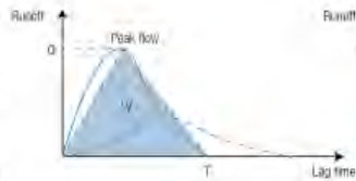
This graph shows, that by increasing the lag time, we can reduce the peak flow and the volume of water generated during a storm. Currently our site generates 60 ac ft in a 100y storm, 34 ac ft in a 5y storm, and 12 ac ft during a 2y storm.
